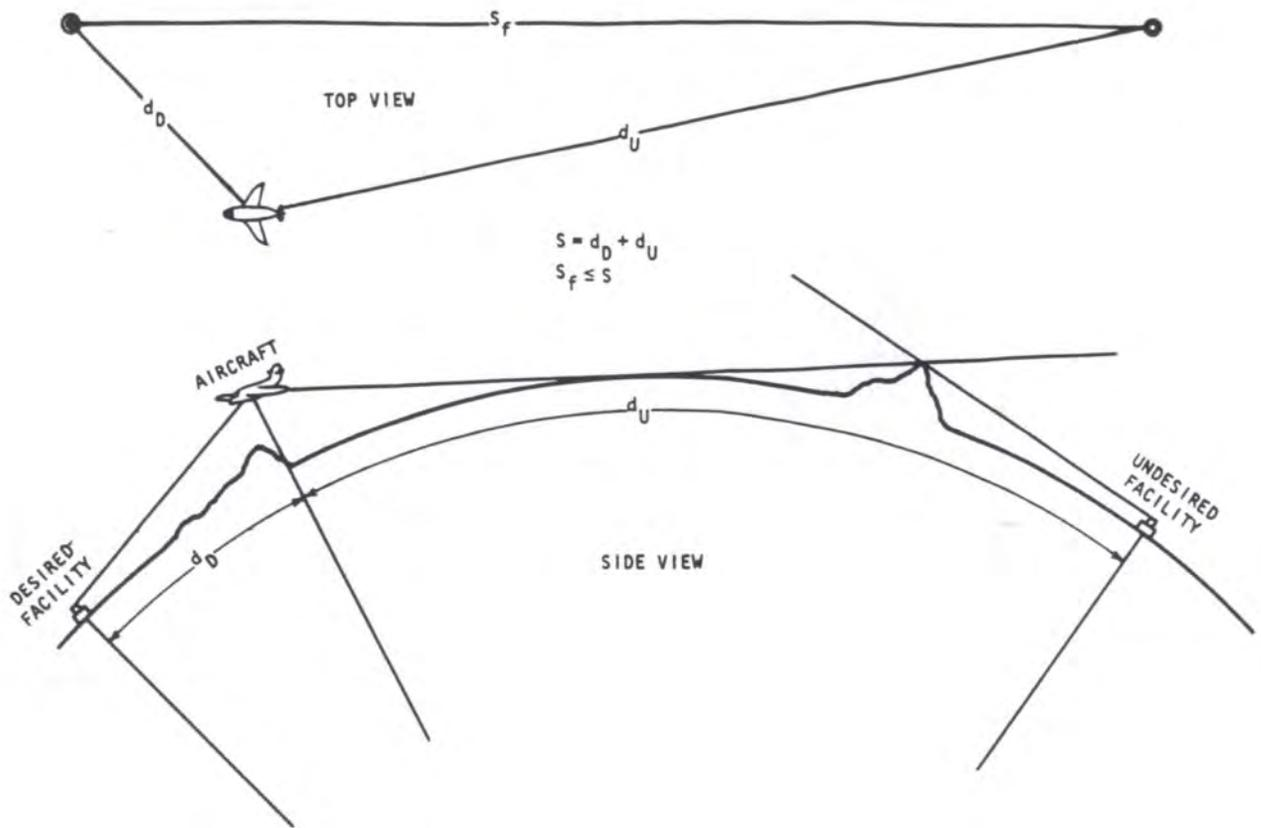
Figure 6. Sketch illustrating interference configuration.
