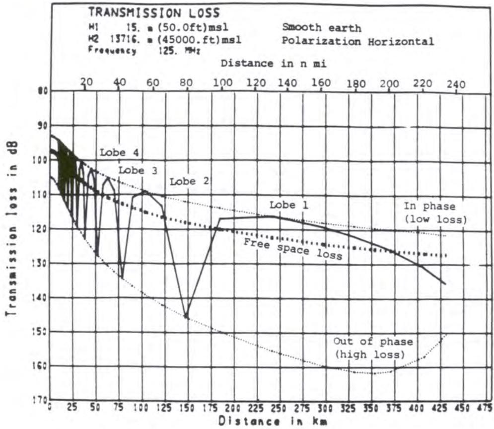
Figure 4. Plot for capability 1, LOBING.
