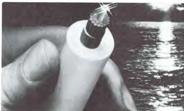
Dawn of a new era. In 1979 this picture was prepared for an advertisement of Bell Laboratories in which it was to be revealed that an experimental glass fiber cable had been under test in a simulated ocean environment at the Holmdel, New Jersey facility of the Laboratories. Tests were at near 0° Celsius and 10,000 pounds per square inch pressure, corresponding to a depth of four miles in the sea. Simplex Wire and Cable Company made the first cable models as designed by Bell Labs.
