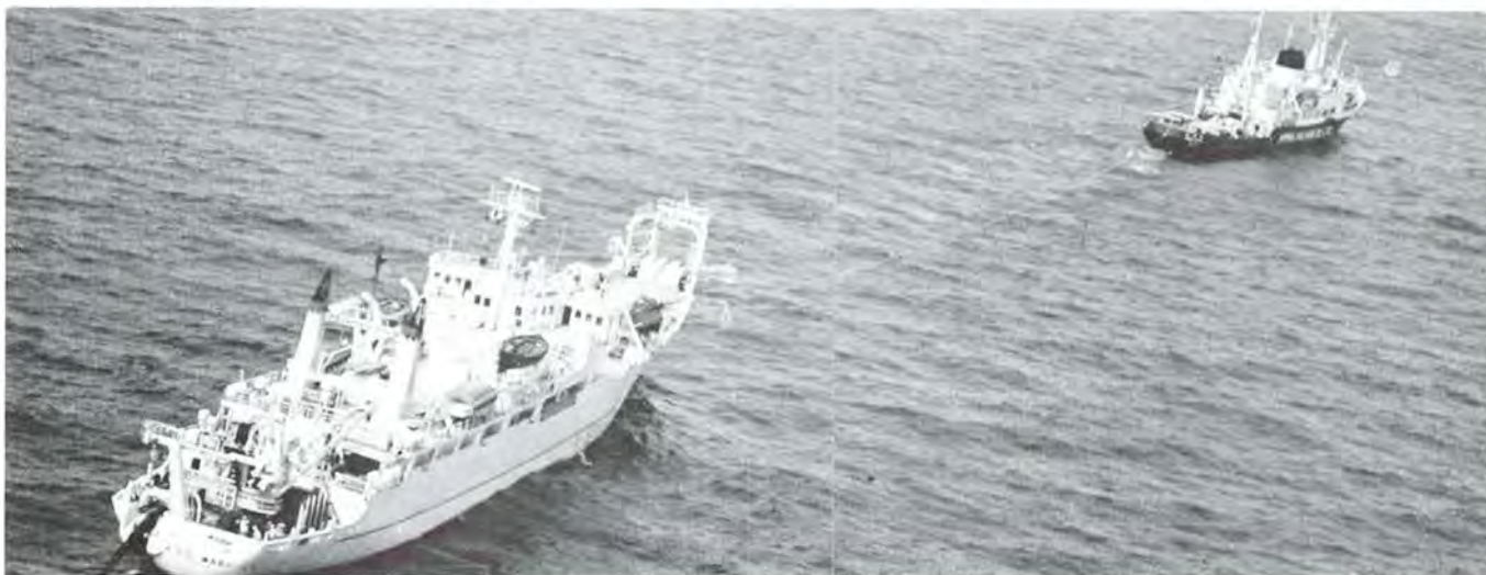
More and more submarine telephone cable projects are turning to cable burial in the sea-floor for reducing the likelihood that the cable will be disturbed by some man-initiated surface activity--trawling, for instance. Here KDD MARU, assisted by a tug, is simultaneously laying and burying the Japan-to-Mainland China cable for the part of the route having depth less than approximately 100 fathoms.
