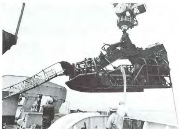
More and more submarine telephone cable projects are turning to cable burial in the sea-floor for reducing the likelihood that the cable will be disturbed by some man-initiated surface activity--trawling, for instance. Here KDD MARU, assisted by a tug, is simultaneously laying and burying the Japan-to-Mainland China cable for the part of the route having depth less than approximately 100 fathoms.
