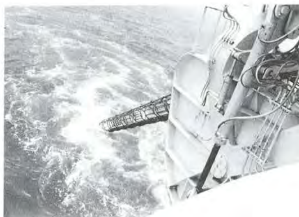
At right, the view from the stern of the ship shows the cage leading from the ship to the plow on the sea-bottom.
