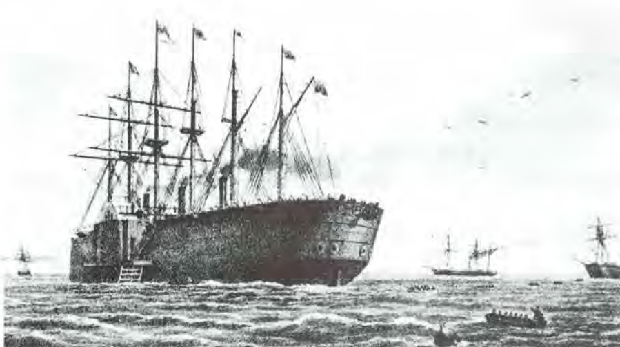
Steamship GREAT EASTERN, then by far the largest ship ever constructed, was converted from her original configuration as a passenger liner to a cable-laying ship and used for attempts to place a telegraph cable between Ireland and Newfoundland. The first success in 1859 was short-lived, the cable failing after only a few weeks in operation. An attempt later, in 1866, resulted in a completely-successful link that operated for many years.
