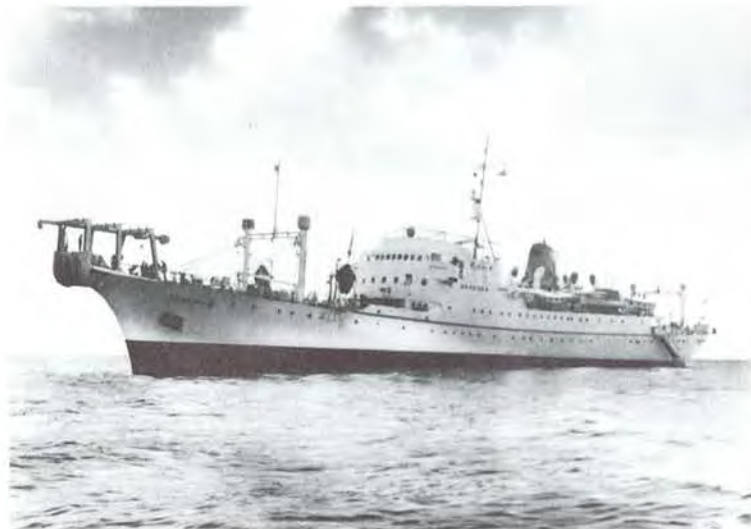
Cablesip LONG LINES, in many respects the world's largest cable-layer, is seen here passing a well-known landmark, Diamond Head, Oahu, Hawaii. Commissioned in 1963, LONG LINES has laid most of the submarine telephone cable systems that land in U.S. territory. Soon she will be elevated to the position of flagship of the AT&T cablesip fleet, as SALERNUM, seen below, just recently acquired by AT&T to supplement the activities of LONG LINES, is undergoing refit and modifications at the Tracor Marine yard in Florida.
