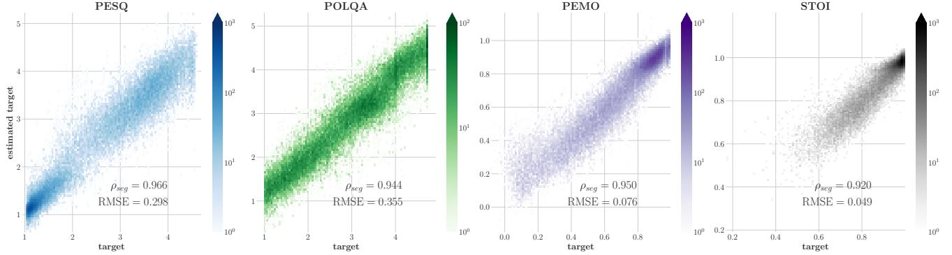
**Fig. 2.** Two-dimensional histograms showing target vs. estimated values for PESQ, POLQA, PEMO, and STOI when evaluated on the unseen dataset. Number of segments per bin is given by the scale at the right.
