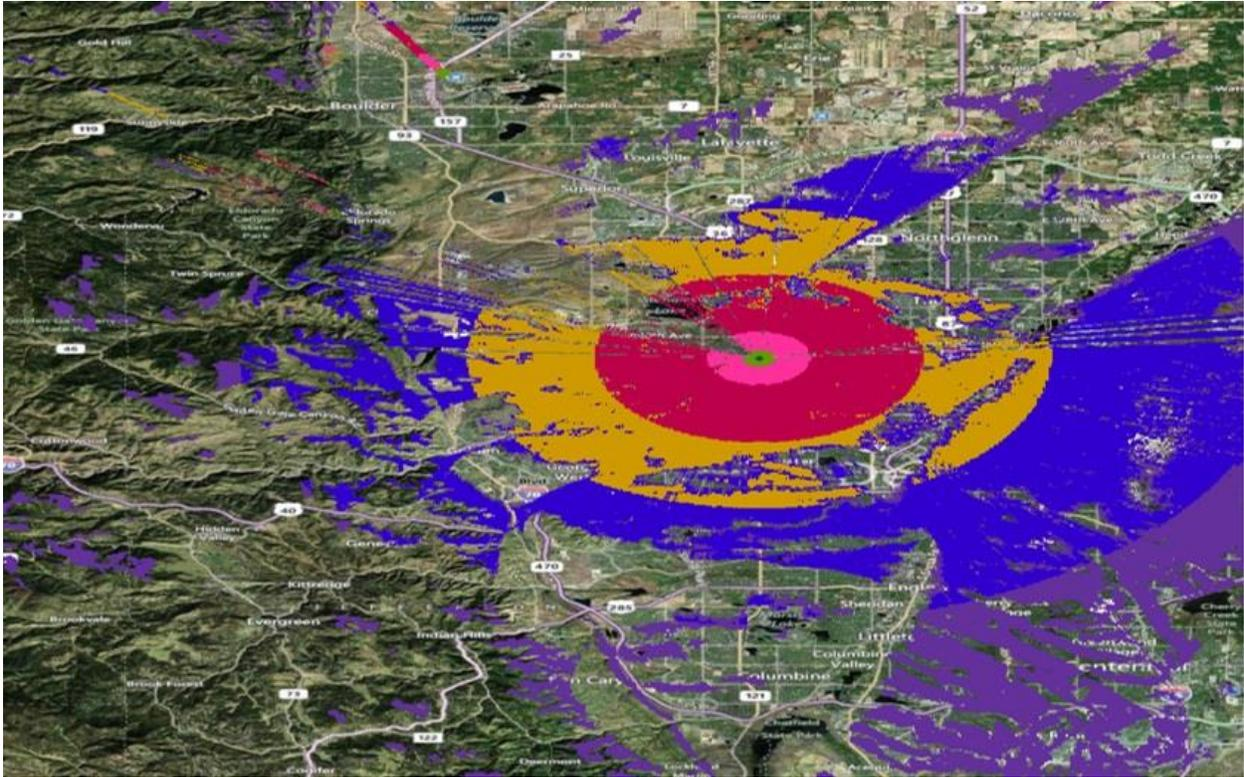
*Figure 2. This field strength study uses the Longley-Rice model for a transmitter located southwest of Boulder, Colorado. The analysis was run in PMW, then imported into GoogleEarth.*
