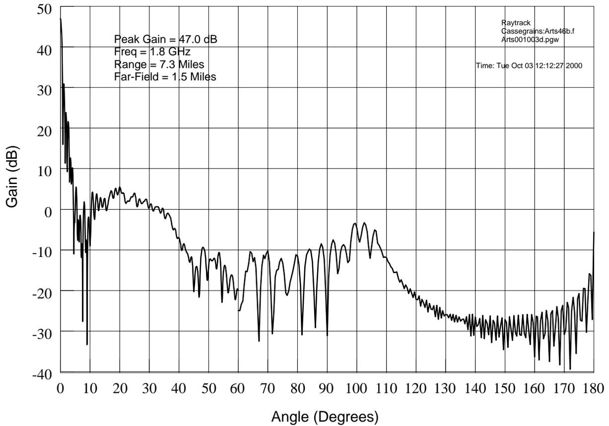
**Figure B-3. Computer Generated Antenna Pattern for the 46-foot Antenna Diameters (Antenna Gain Values are in dBi)**
