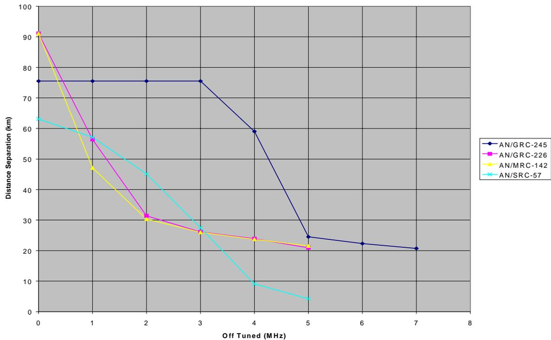
Figure C-2. Frequency-Distance Separation for IMT-2000 GSM to TRR
