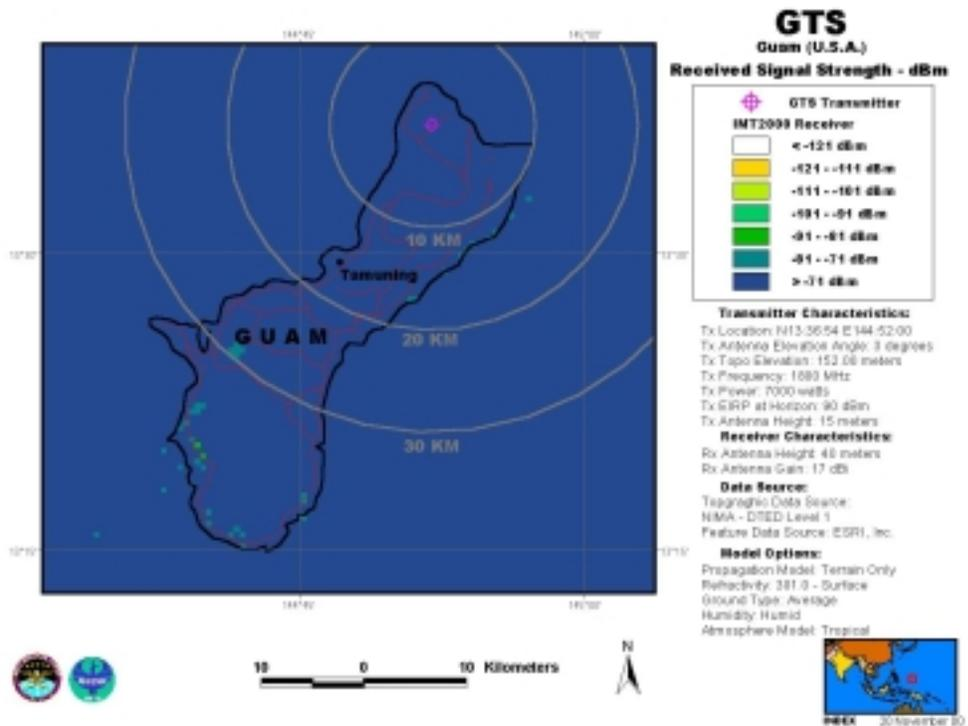
GTS, Antenna Elevation Angle: 3°, Transmitter Power: 7000 W, IMT-2000 Base Station
