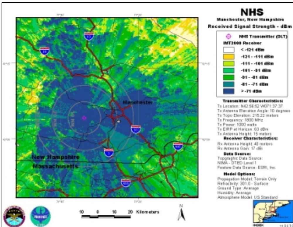
NHS-DLT, Antenna Elevation Angle: 10°, Transmitter Power: 1,000 W, IMT-2000 Base Station
