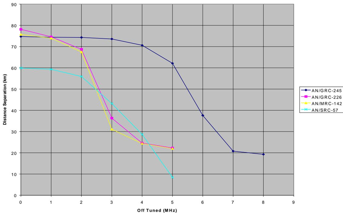
Figure C-1. Frequency-Distance Separation for CDMA-WB to TRR
