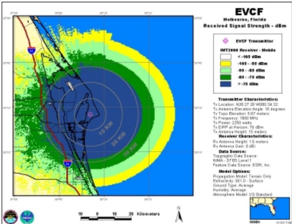
EVCF, Antenna Elevation Angle: 10°, Transmitter Power: 2,250 W, IMT-2000 Mobile Station
