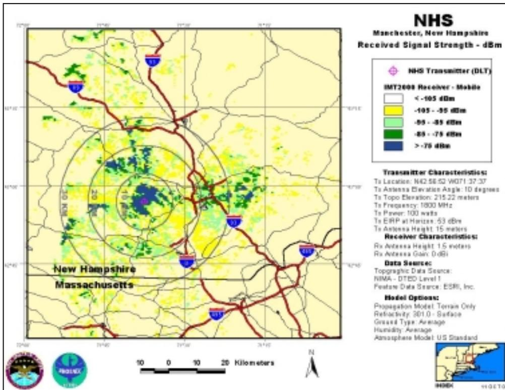
NHS-DLT, Antenna Elevation Angle: 10°, Transmitter Power: 100 W, IMT-2000 Mobile Station
