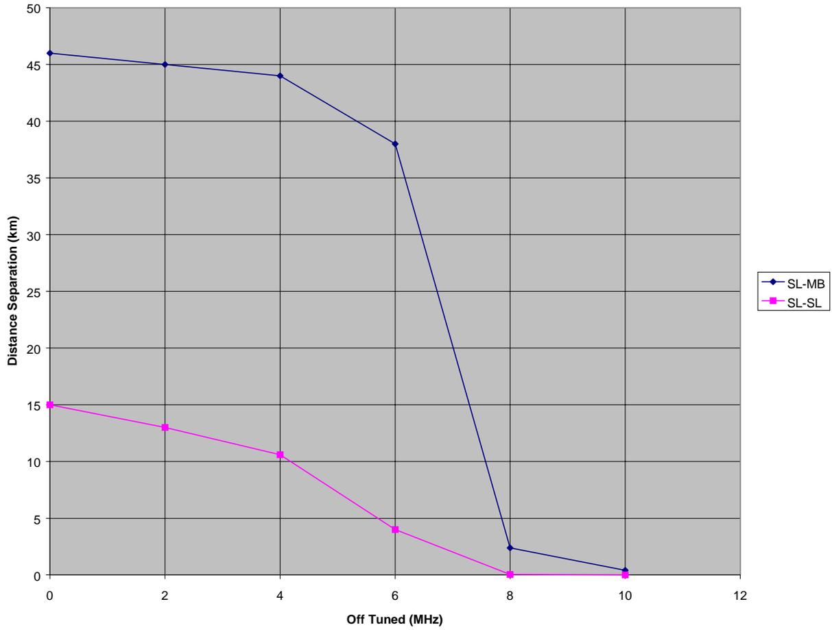
Figure C-11. Frequency-Distance Separation for AN/GRC-222 to a TRR
