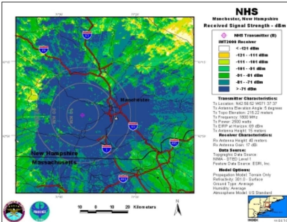
NHS-B, Antenna Elevation Angle: 5°, Transmitter Power: 2,500 W, IMT-2000 Base Station
