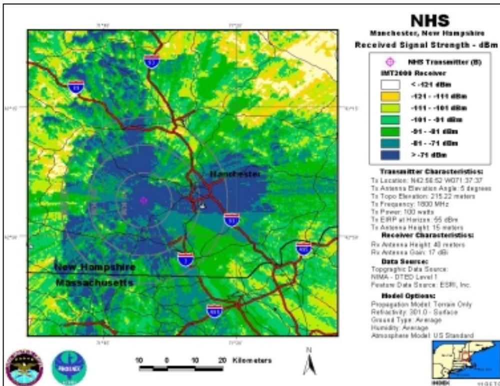
**NHS-B, Antenna Elevation Angle: 5°, Transmitter Power: 100 W, IMT-2000 Base Station**
