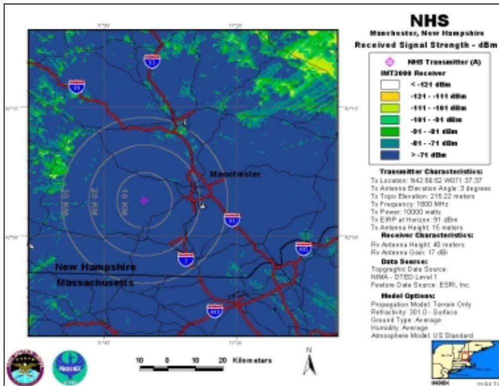
NHS-A, Antenna Elevation Angle: 3°, Transmitter Power: 10,000 W, IMT-2000 Base Station
