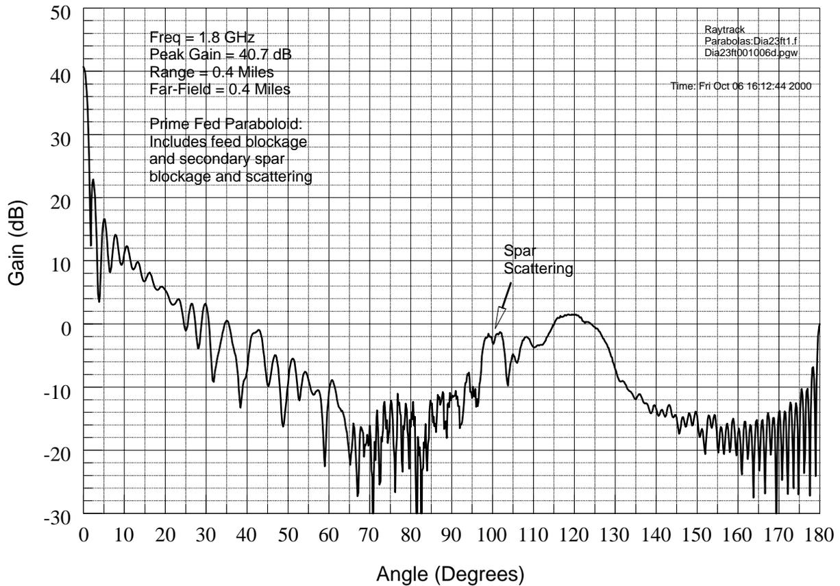
Figure B-5. Computer Generated Antenna Patterns for the 23-Foot Antenna Diameters (Antenna Gain Values are in dBi)
