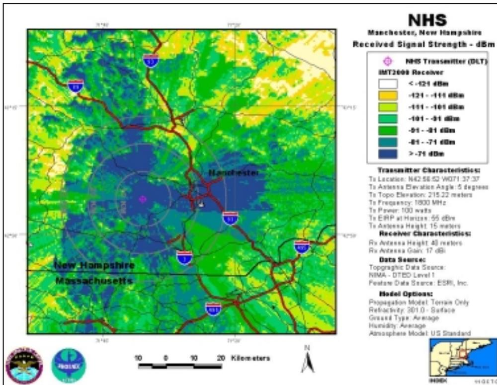
**NHS-DLT, Antenna Elevation Angle: 5°, Transmitter Power: 100 W, IMT-2000 Base Station**
