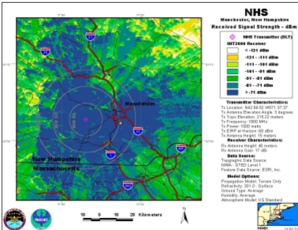
NHS-DLT, Antenna Elevation Angle: 3°, Transmitter Power: 1,000 W, IMT-2000 Base Station
