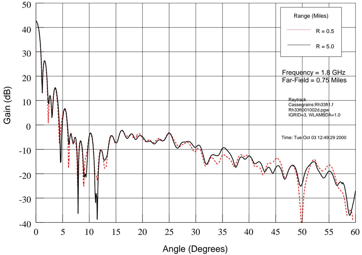
**Figure B-4. Computer Generated Antenna Patterns for the 33-Foot Antenna Diameters (Antenna Gain Values are in dBi)**
