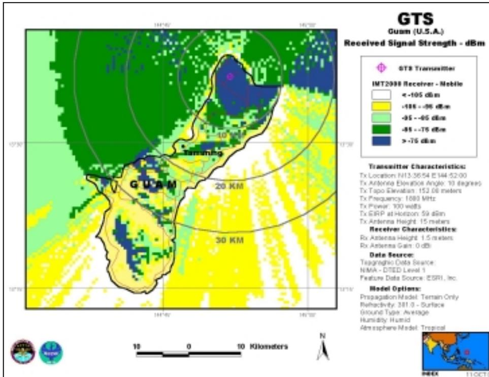
GTS, Antenna Elevation Angle: 10°, Transmitter Power: 100 W, IMT-2000 Mobile Station
