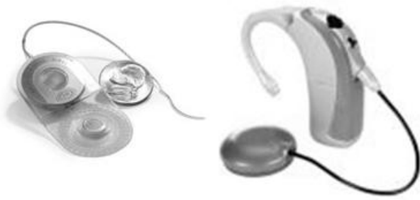
Figure 2. Cochlear implant and external speech processor.
