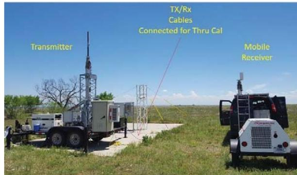
Fig. 11. Channel sounder thru calibration at the transmitter site.
