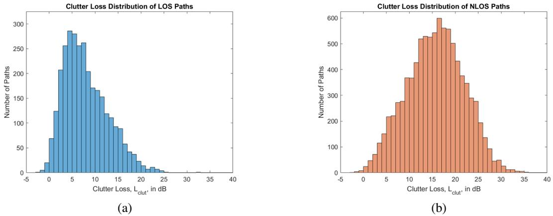
Fig. 4. Distribution of clutter loss (a) for line-of-sight (LOS) and (b) non-line-of-sight (NLOS) measurement data points.
