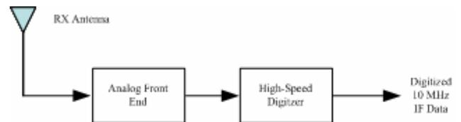
Figure 5. Receiver system architecture
