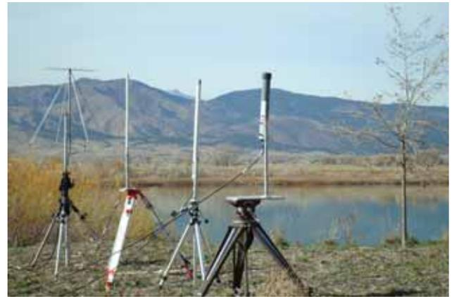
Figure 4. Group 2 transmitting antennas deployed at a rural site.
