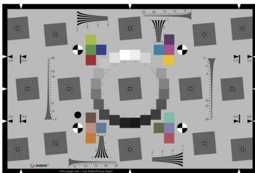
Figure 1. This eSFR ISO chart from Imatest implements the ISO 12233:2014 standard, with some added features. See [http://www.imatest.com/docs/esfriso\\_instructions/](http://www.imatest.com/docs/esfriso_instructions/)
