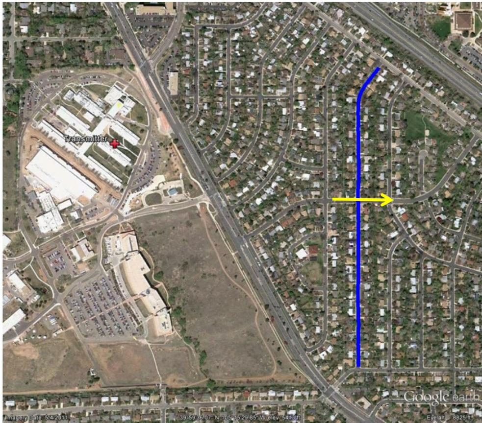
Figure 40. NLOS drive path in Martin Acres next to the Boulder Laboratories. The transmitter is shown by the red + and the street chosen for analysis is shown by the blue line. The yellow arrow is the location of a wave-guiding street.
