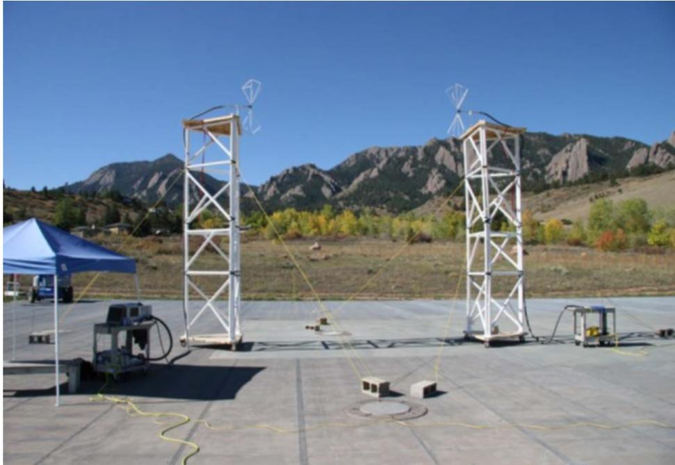
Figure B-2. Photo of an antenna measurement at the NIST OATS facility at the Boulder Laboratories.
