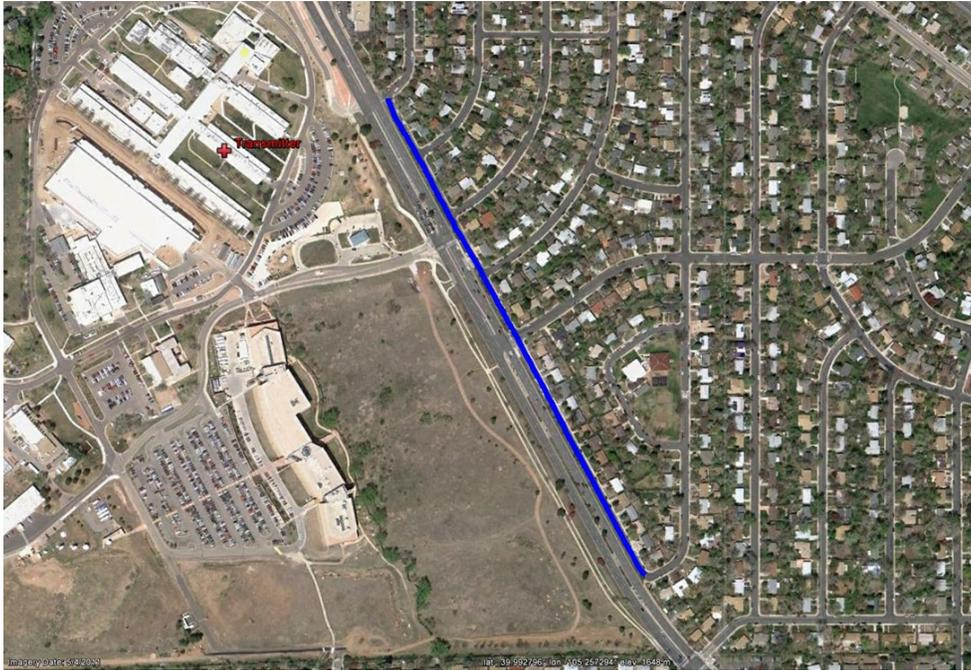
Figure 46. LOS drive path in Martin Acres next to the Boulder Laboratories. The transmitter is shown by the red + and the street chosen for analysis is shown by the blue line.
