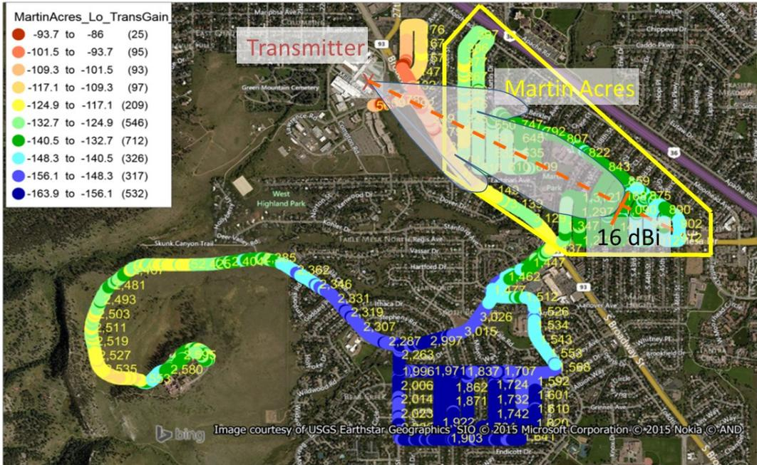
Figure 23. Using a directional antenna to make measurements in the Martin Acres neighborhood.
