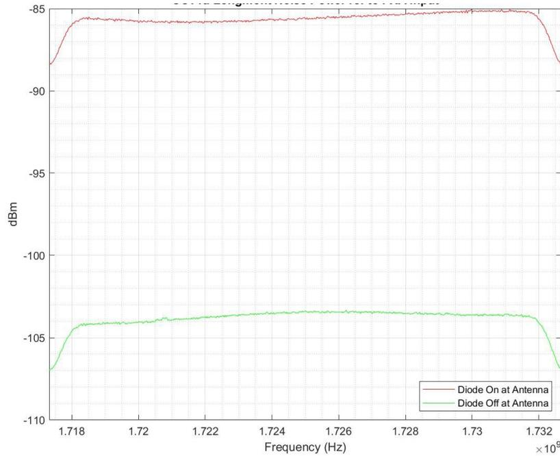
Figure 7. Noise power measurements over the total capture bandwidth.
