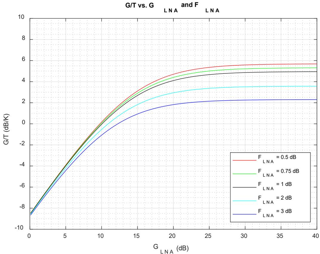
Figure 3. G/T assuming a fixed antenna gain but varying LNA gain and noise figure.
