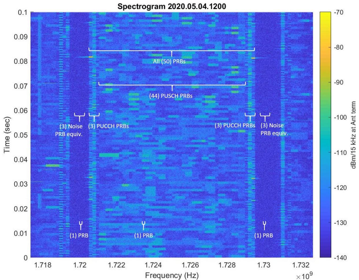
Figure 9. Spectrogram showing 100 ms of LTE UE uplink activity and channelization
