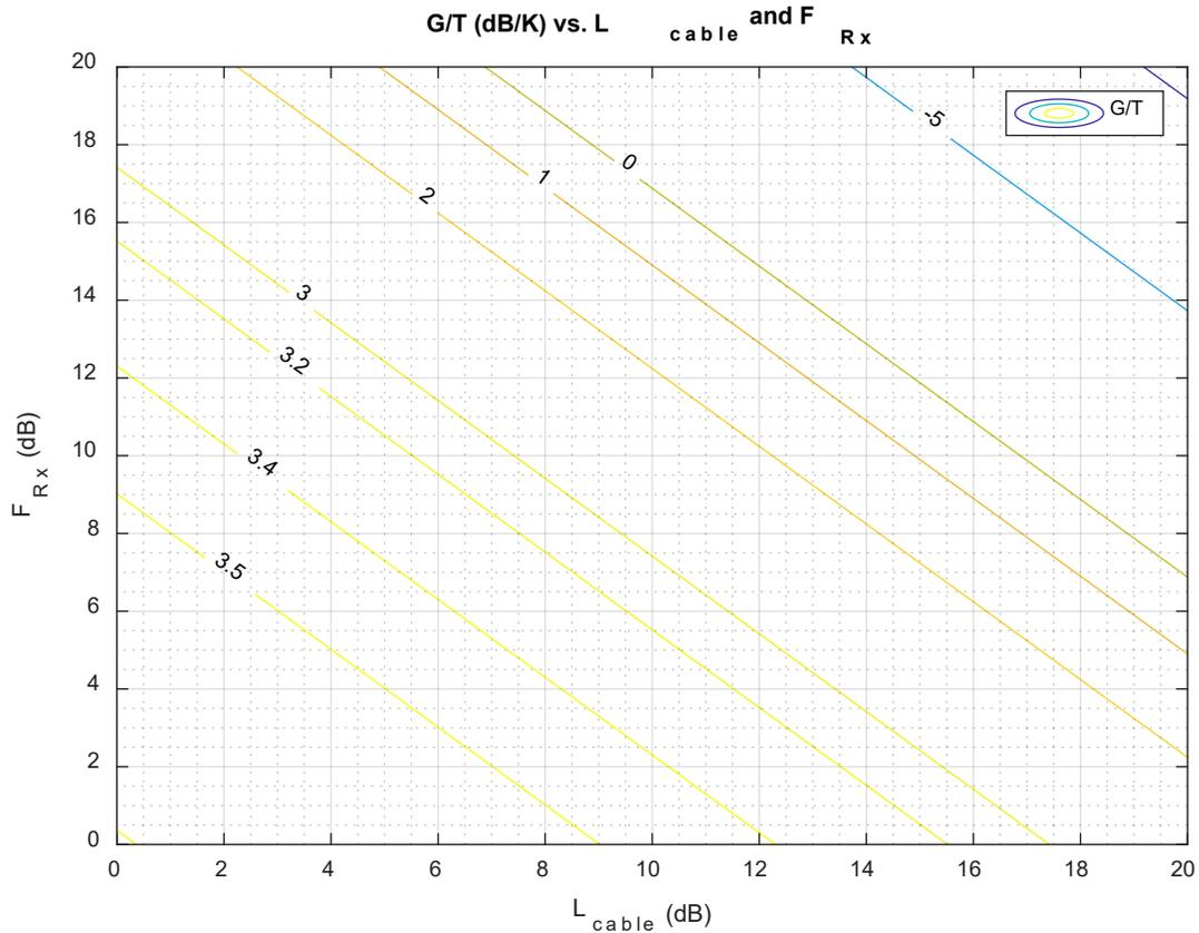
Figure 5.  $G/T$  contour plot for various receiver noise figures and cable losses.
