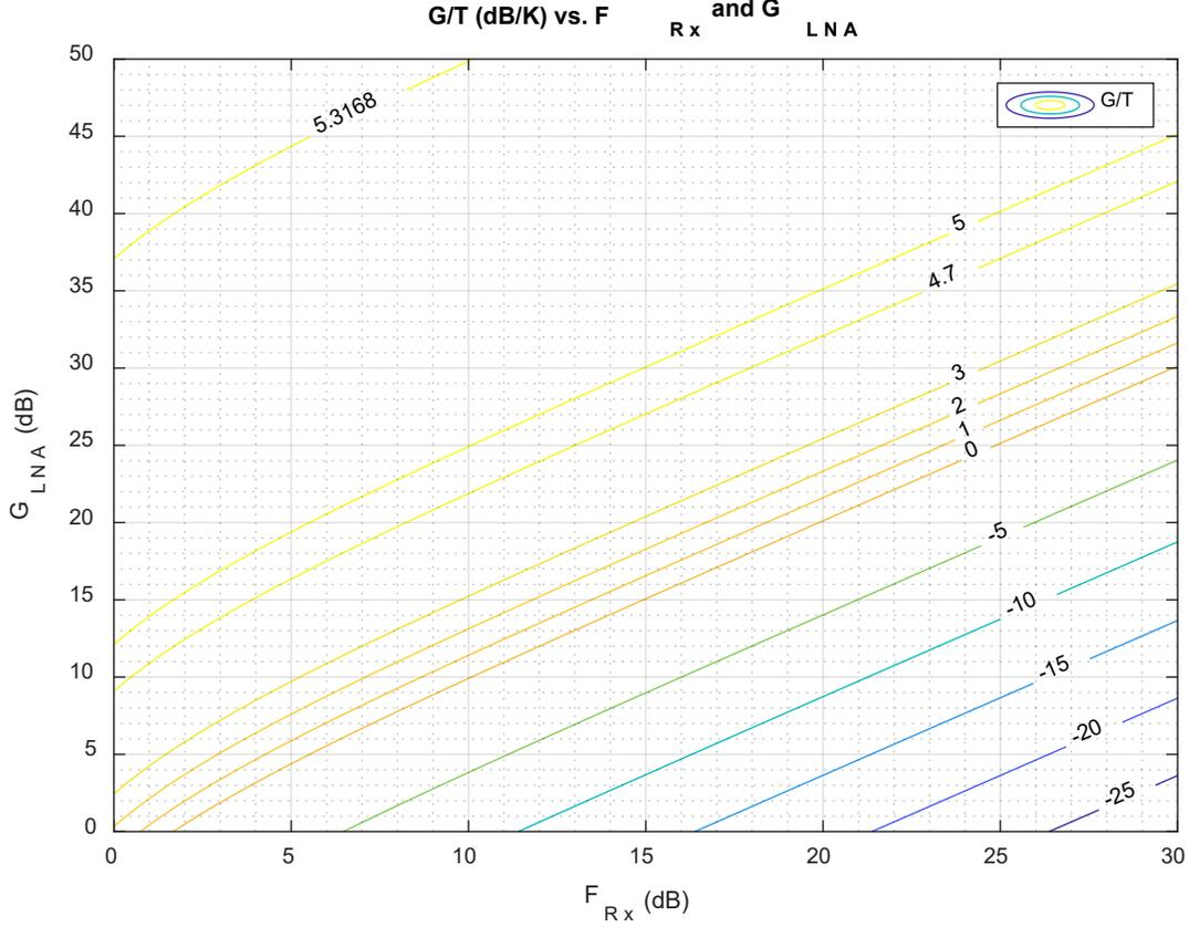
Figure 4. G/T contour plot for various receiver noise figures and LNA gains.
