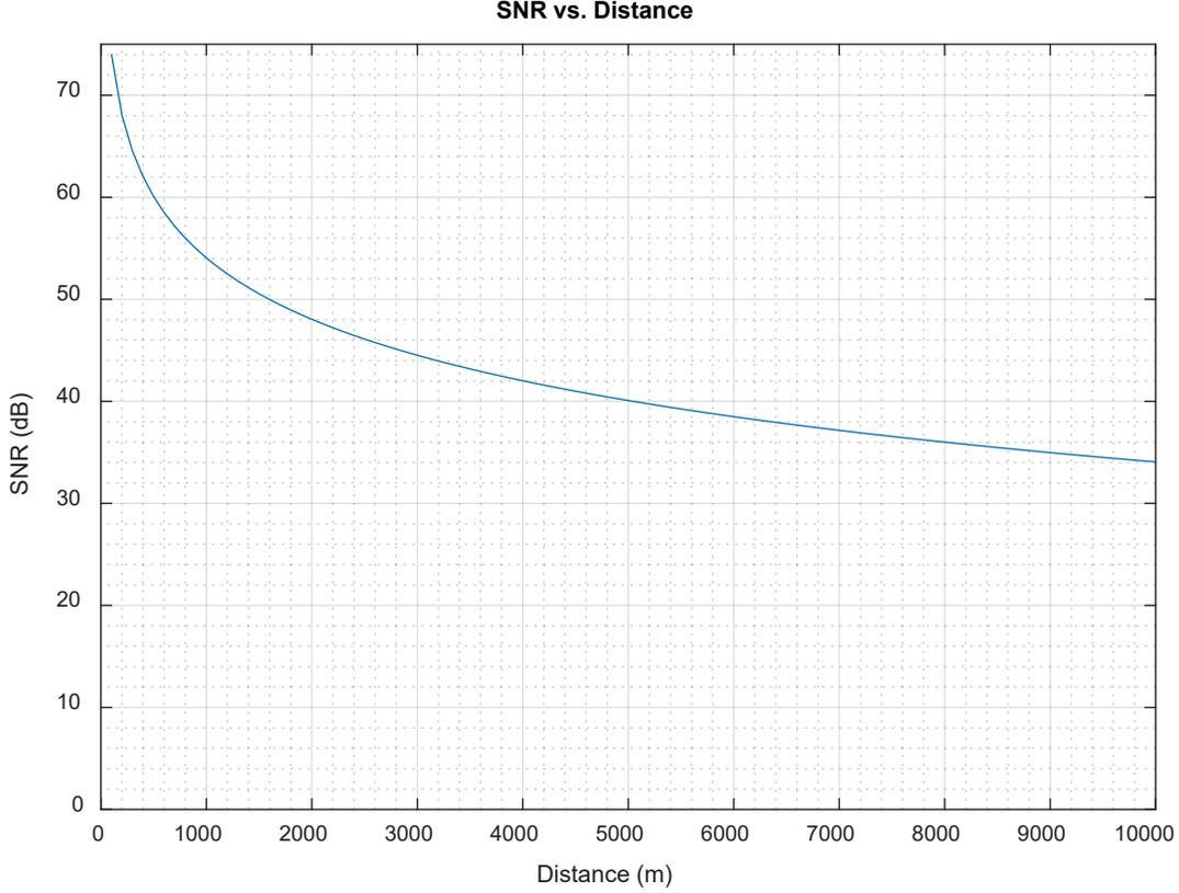
Figure 2. *SNR vs. distance* for a simplified scenario where  $f = 1745$  MHz,  $B = 15$  kHz, and  $EIRP = -30$  dBW in a 180 kHz bandwidth
