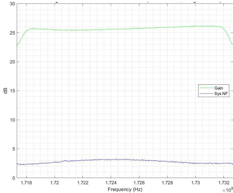
Figure 8. System gain and noise figure over the total capture bandwidth.
