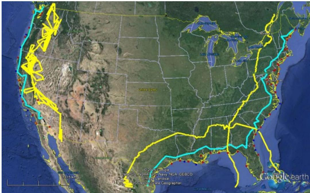
Figure B-19. Shipborne Radar 5–Exclusion zone lower 48 states (yellow line–fast track exclusion zone and blue line–revised exclusion zone).
