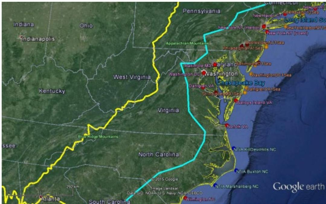
Figure B-24. Shipborne Radar 5–Exclusion zone middle east coast (yellow line–fast track exclusion zone and blue line–revised exclusion zone).
