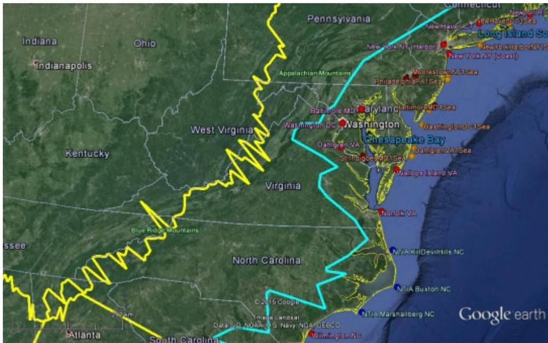
Figure B-15. Shipborne Radar 4–Exclusion zone middle east coast (yellow line–fast track exclusion zone and blue line–revised exclusion zone).
