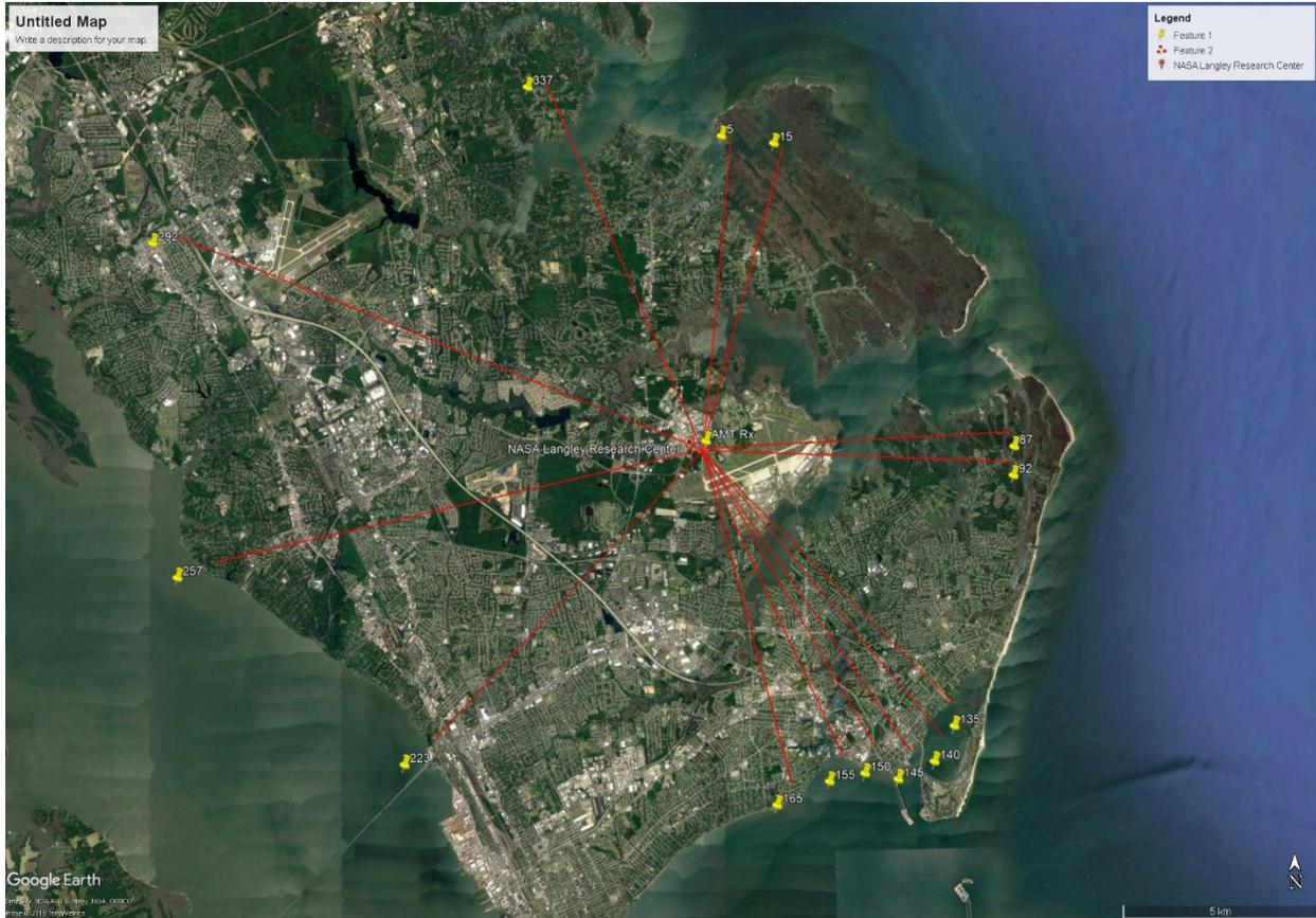
Figure 10. Key azimuths traced to potential sources from which strong emissions were observed at NASA/LaRC.
