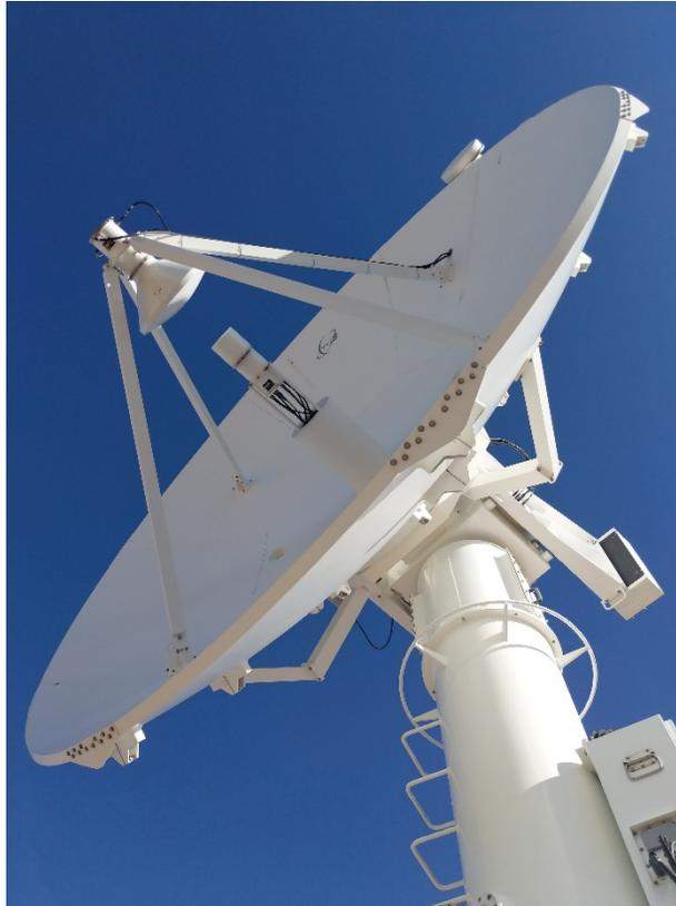
Figure 2. Antenna 5 at the EAFB collection site. The sealed feed sections were inaccessible for noise diode based calibration procedures, thus a gain over thermal noise (G/T) measurement was performed.
