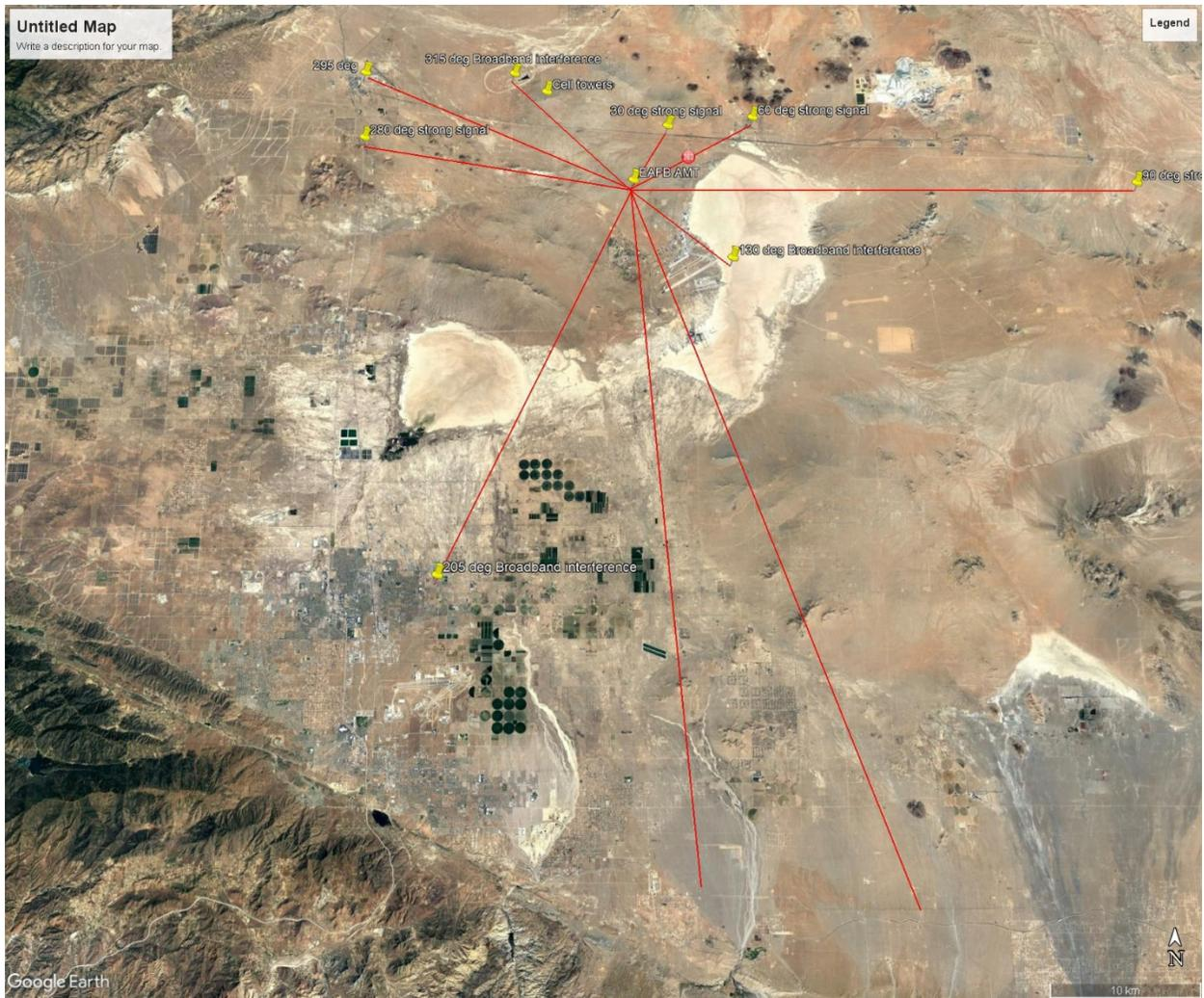
Figure 9. Key azimuths traced to potential sources from which strong emissions were observed at EAFB.
