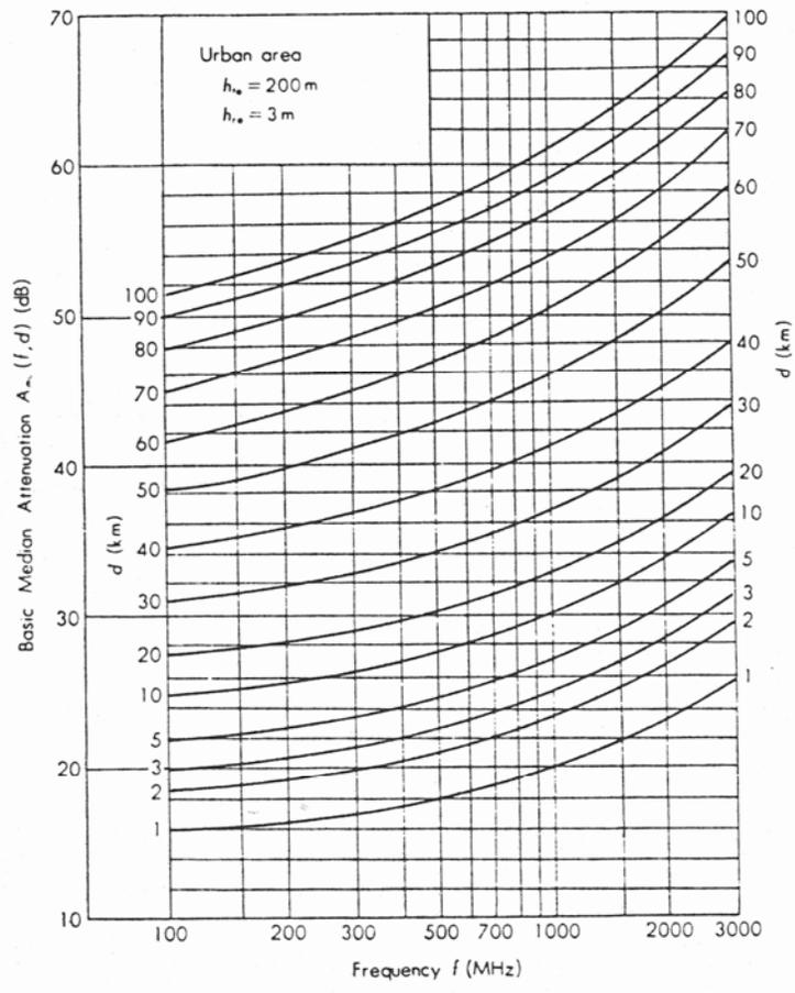
Figure 1. Prediction curve for basic median attenuation relative to free space in urban area over quasi-smooth terrain, referred to  $h_{te} = 200\text{ m}$ ,  $h_{re} = 3\text{ m}$ . From Okumura et al. (1968).
