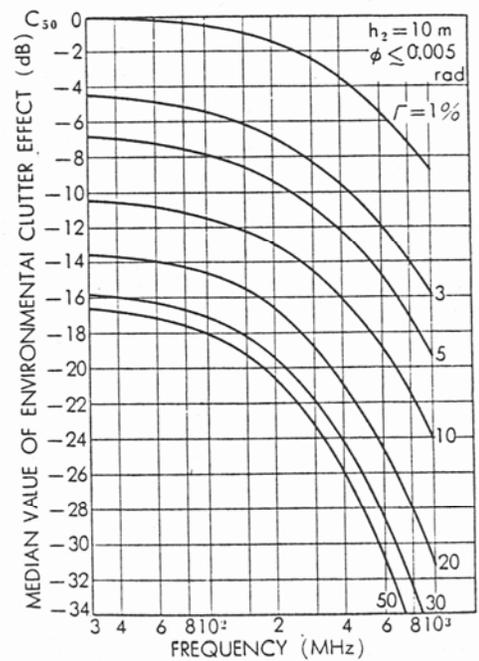
Figure 3. Median value of clutter effect as a function of frequency. From Kinase (1969).
