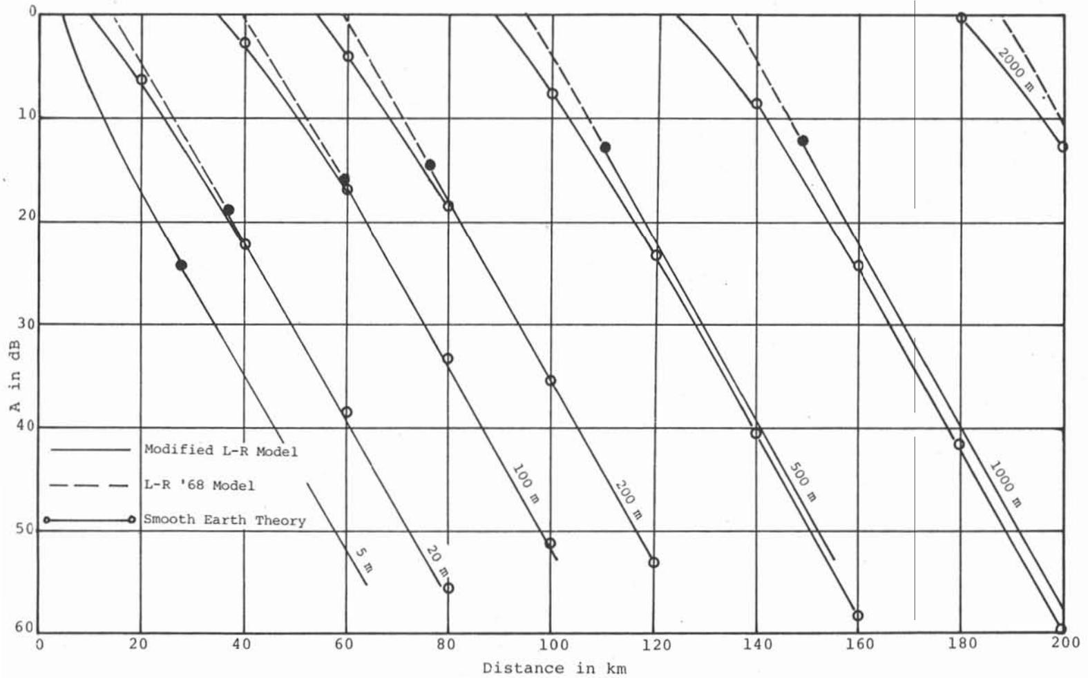
Figure A-4. Attenuation relative to free space as a function of distance over a smooth homogeneous earth. Frequency 1000 MHz,  $\epsilon = 15$ ,  $\sigma = 5$  mS/m,  $h_1 = 20$  m,  $h_2 = 5$  to 2000 m.
