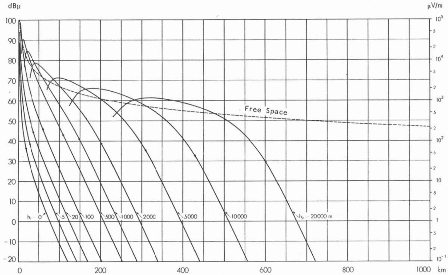
Figure A-1. Field strength (for 1 kW ERP) as a function of distance over a smooth homogeneous earth. Frequency 100 MHz,  $\epsilon = 10$ ,  $\sigma = 10$  mS/m,  $h_1 = 20$  m,  $h_2 = 0$  to 20,000 m.
