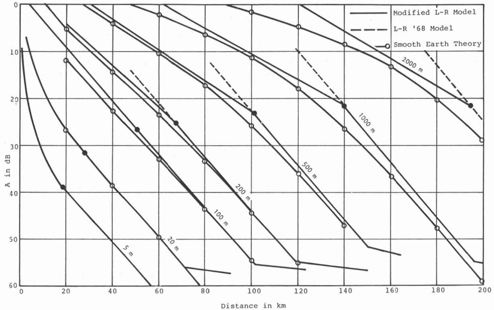
Figure A-3. Attenuation relative to free space as a function of distance over a smooth homogeneous earth. Frequency 300 MHz,  $\epsilon = 15$ ,  $\sigma = 5$  mS/m,  $h_1 = 5$  m,  $h_2 = 5$  to 2000 m.
