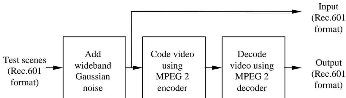
Figure 1. Block diagram for generating subjective test material.
