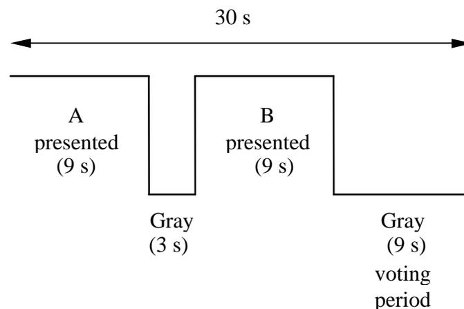
**Figure 4. Layout of each clip pair on the video tape.**
