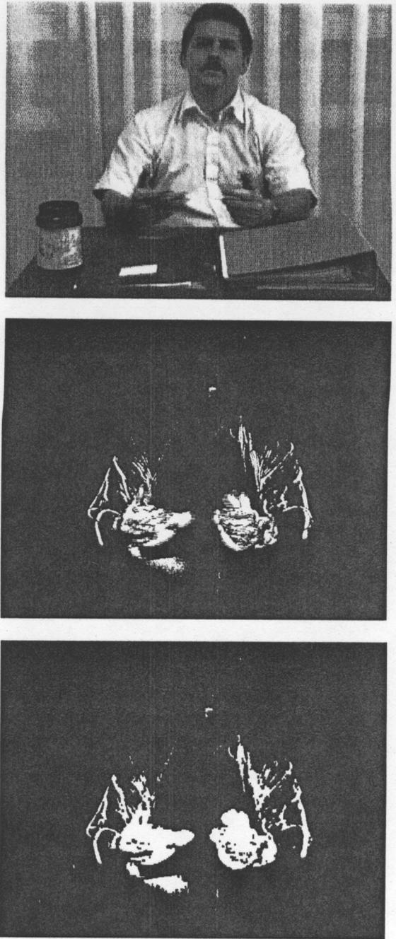
Figure 6. The performance of the motion-still segmentation algorithm for arm and hand motion. Top - original input image. Middle - binary difference image. Bottom - motion mask.
