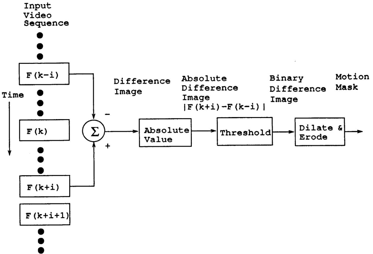
Figure 1: Motion-Still Algorithm Conceptual Block Diagram
